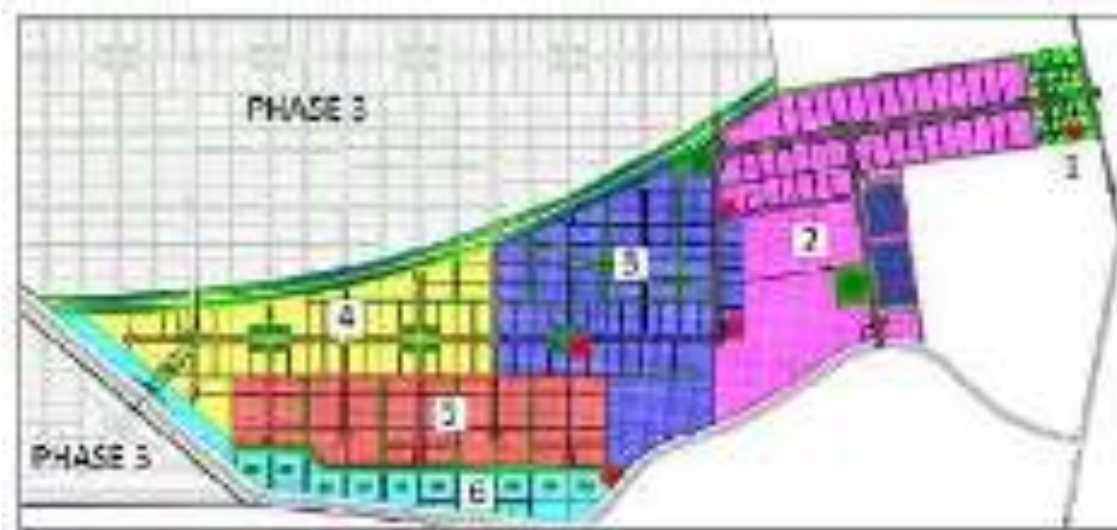
Figure 18: Water supply zones for Phase 1 and 2
